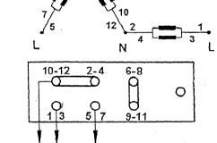
50 Hz L-L 230 volts 50 Hz L-N 115 volts 60 Hz L-L 277 volts 60 Hz L-N 138 volts (Refer to Note #1)
