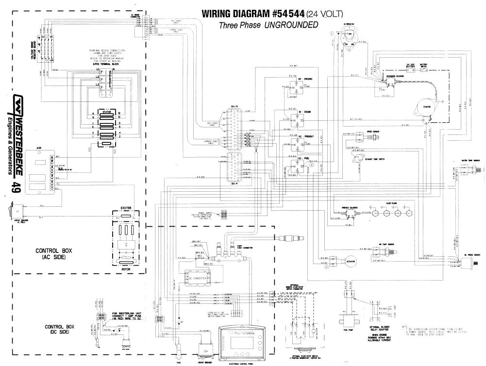
WIRING DIAGRAM #54544 (24 VOLT) Three Phase UNGROUNDED
