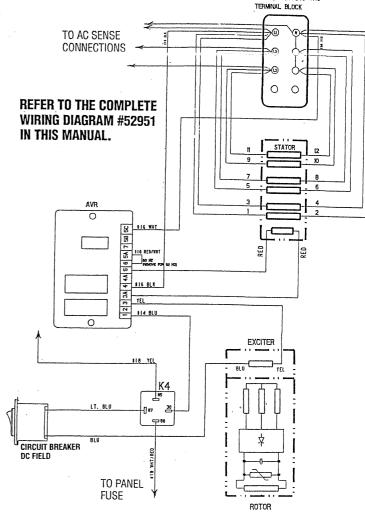
TERMINAL BLOCK CONNECTIONS SHOWN ARE CONFIGURED FOR LO-WYE 120/208 VAC
